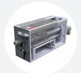
**GM SmartSlit** - automatically positions up to 16 knives in 2 minutes, saving valuable time on short run jobs.
