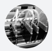
**GM SmartCrush** - An ultra-quick set knives system, allowing fast and precise setting of each crush knife – also while running.
