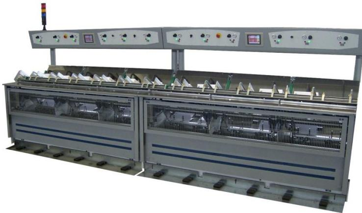
It is possible to load two different signatures in a sequential order into the same pocket gatherer if the signatures to gather have a maximum size head to tail no more than 320mm (patented). So the dimensions of the complete line is REDUCED, the loading/unloading operation made by ONLY ONE OPERATOR NECESSARY to the line functioning is facilitated.
