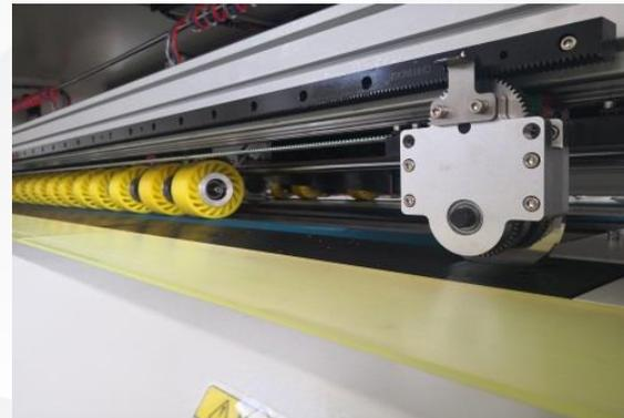
Powered horizontal trimming knife
