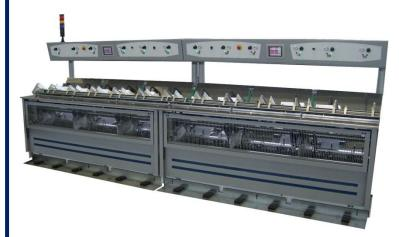
In case of the signature book number are more than the stations gatherer available, the UNIT LINE is equipped with an HAND FEEDING STATION (Standard) to feed manually a PRE GATHERED signature block.
