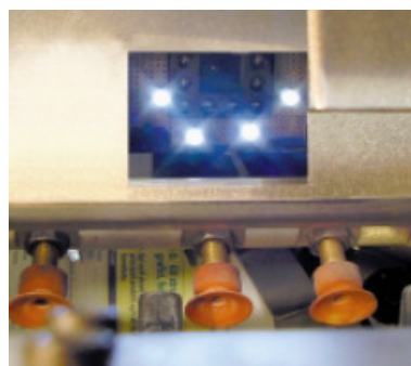
New camera control of the correct gathering sequence in the hopper (option)
