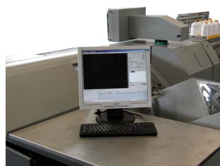
New camera control of the correct gathering sequence in the hopper (option)
